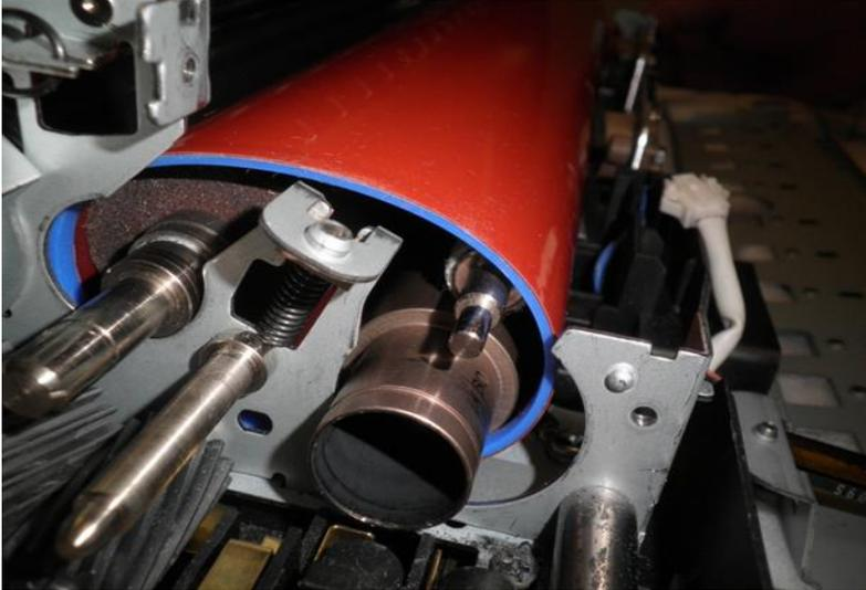
21. Lift the ends of the tensioner roller and place in the bushings:
