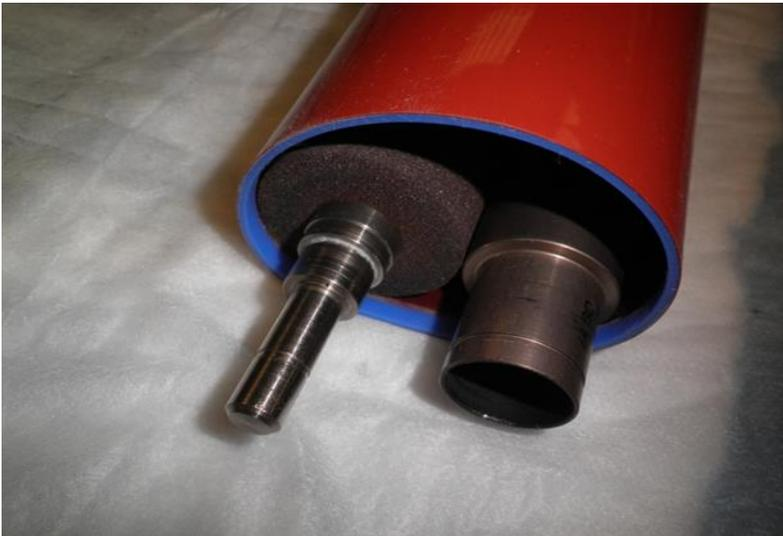
18. Grasping the ends of the heat roller, drop the foam pressure roller into its frame opening:
