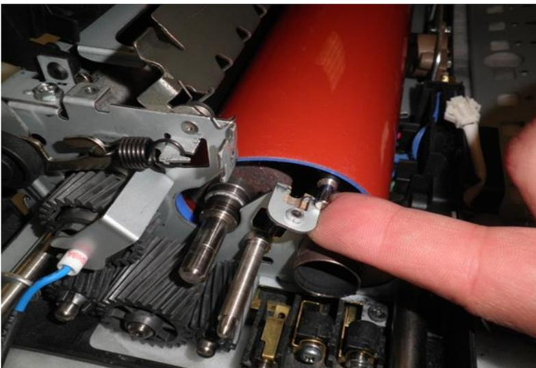
22. Move the foam pressure roller toward the drive side so that the larger diameter is resting on the frame:
