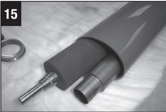
■ Place foam pressure roller and heat roller inside new belt.
