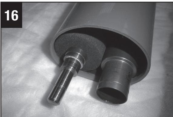
■ Align large diameters of rollers inside of guide ribs.
