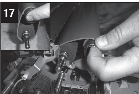
■ Grasping the ends of the heat roller, insert the foam pressure roller into its frame opening.
